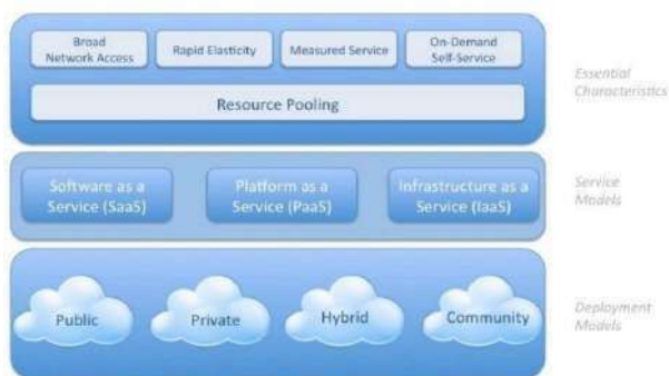
Fig. 2. NIST Visual Model of Cloud Computing Definition.
